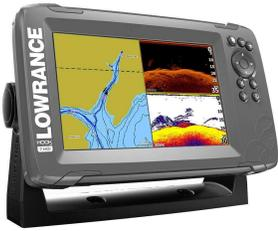
I just purchased a Lowrance Hook 2 Fish locator. Like most new models they have a number of features that my old one didn't. One of the more interesting is Side Imaging. This imaging provides picture like images of structure on the bottom of the lake on each side of the boat. Right now, my is set to out 50 feet to the right and left of the boat.
